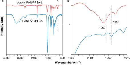
(a) FT-IR spectra and (b) a magnified view of the spectra of PAN/PVP/PFSA and porous PAN/PFSA-Li.
