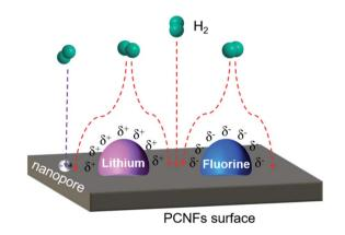
Fig. 8 The mechanism of hydrogen adsorption by the Li-F-PCNFs composites.
