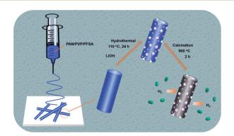
Fig. 1 The fabrication procedure for the Li-F-PCNFs composites.
