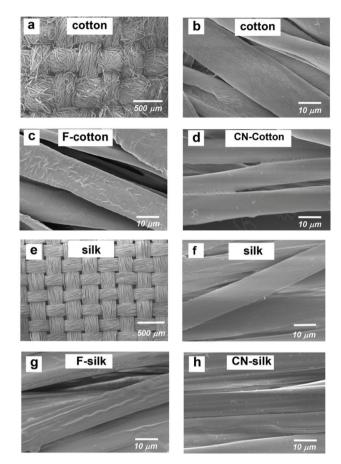
Fig. 2 (a) and (b) SEM images of plain cotton (500x) and (2000x), (c) fluoroalkylated siloxane coated cotton (F-cotton) (2000x), (d) cyanoalkylated siloxane coated cotton (2000x) (CN-cotton); (e) and (f) SEM images of plain silk (500x) and (2000x), (g) fluoroalkylated siloxane coated silk (F-silk) (2000x) and (h) cyanoalkylated siloxane coated silk (CN-silk) (2000×).
