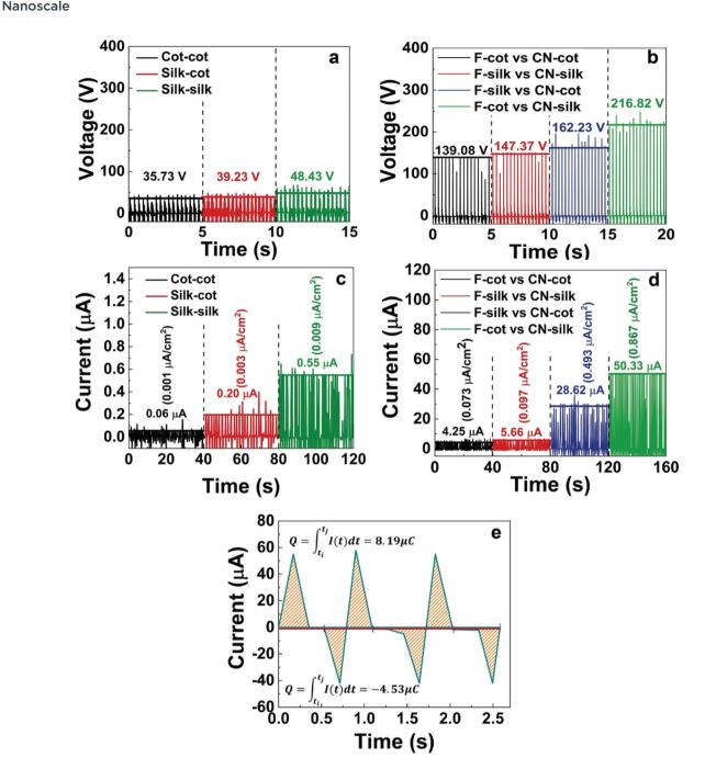
Fig. 6 (a) Output voltage of pristine-TENGs, (b) output voltage of N-TENGs, (c) output current of pristine-TENGs, (d) output current of N-TENGs and (e) three movement cycles of the  $I_{sc}$  signal of F-cot/CN-silk with the average calculated surface charge.
