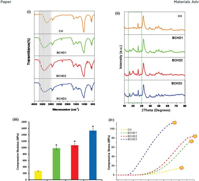
Fig. 1 FTIR spectra (i), XRD diffractograms (ii), mechanical strength analysis: compressive modulus (iii), and compressive stress-strain (iv) curves of BCHD1, BCHD2, BCHD3 and CH nanocomposite scaffolds where the fracture point has been shown by yellow color, \*p < 0.05 showing the statistical difference compared with the CH nanocomposite scaffold
