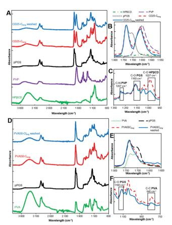
Fig. 4 ATR-FTIR spectra of CD25 (A–C) and PVA50 (D and E) after curing and after purification compared to HPβCD, PVP, PVA and corresponding pPGS spectra. (A and D) Full spectra. (B and E) C=O bands, absorbance normalized to the 1730 cm $^{-1}$  band. (C and F) C=O, C=C and C=N bands, absorbance normalized to the 1160 cm $^{-1}$  band.
