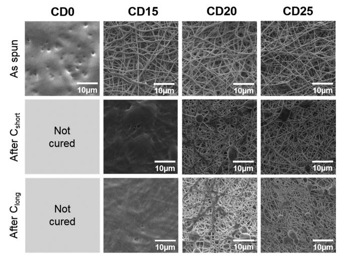
Fig. 2 Influence of the proportion of HPβCD on the PGS/HPβCD/PVP fiber morphology before and after curing for various formulations. CD0 contains 50% of PGS and 50% of PVP; CD15 contains 50% of PGS, 15% of HPβCD and 35% of PVP; CD20 contains 50% of PGS, 20% of HPβCD and 30% of PVP. The morphology is shown after the following curing steps: 24 h at 120 °C followed by 48 h at 140 °C ( $C_{short}$ ) or 24 h at 120 °C, 48 h at 140 °C and 24 h at 170 °C ( $C_{long}$ ).
