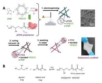
Fig. 1 Strategy for the elaboration of the elastomeric PGS-based fibers. During thermal treatment, pPGS is crosslinked and reaction of -OH groups of HPBCD with -COOH groups of pPGS (in red) occurs (A). Chemical scheme of pPGS synthesis by polycondensation of glycerol and sebacic acid (B)
