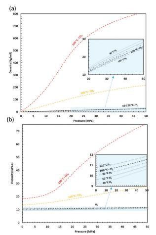
Fig. 4 Density and viscosity of hydrogen,  $CO_2$  and  $CH_4$ . The variation of hydrogen density and viscosity as a function of pressure at different temperatures together with a comparison between the densities of hydrogen,  $CH_4$  and  $CO_2$  at 100 °C.
