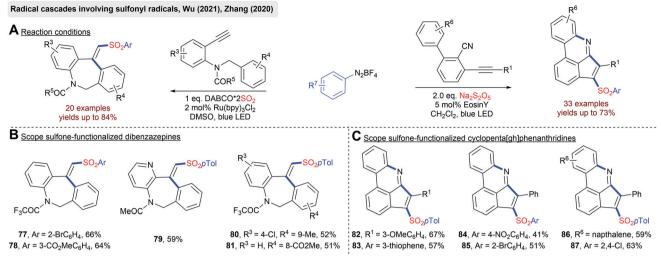
Scheme 19 Photoredox-catalyzed cascades towards sulfonylated heterocycles
