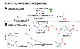
Scheme 7 Electrochemical synthesis of perfluoroalkylsulfinic acids; [a]: DMF/H $_2$ O (9:1), 20 °C, carbon fiber electrodes, divided cell (glass frit), 1–12 mA cm $^{-2}$  (galvanostatic),  $\sim$ 1.05 F; [b]: yield determined by NMR integration ( $^{19}$ F NMR).
