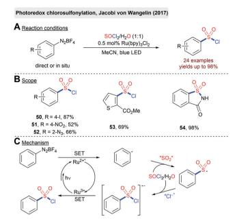
Scheme 13 Photoredox-catalyzed synthesis of sulfonyl chlorides.
