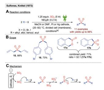
Scheme 4 Electrochemical synthesis of symmetric sulfones; [a]: potentiostatic conditions: -0.7 V vs. Ag/AgCl, 1 F mol<sup>-1</sup> or galvanostatic conditions: 300 mA cm $^{-2}$  and 500 mA cm $^{-2}$ , 2000–10000 C.
