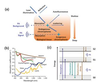
Fig. 1 (a) Schematic diagram of the interaction between light and tissue caused by the excitation light. (b) Absorption spectra of the main endogenous chromophores: oxyhemoglobin, red line; deoxyhemoglobin, green line; water, blue line; lipids, yellow lines; melanin, brown line; and collagen, black line. Adapted from ref. 22. Copyright © 2019 Springer Link. (c) Schematic diagram of photoacoustic signal generation
