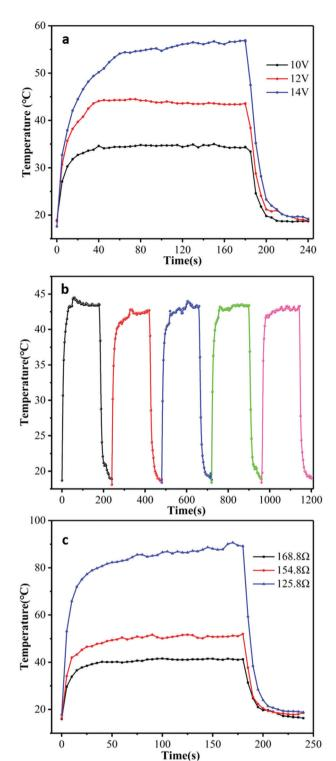
Fig. 4 (a) Temperature profiles of the GNP fabric at different  $V_{\rm GNP}$ ; (b) temperature response of the GNP fabric over 5 cycles at  $V_{\rm GNP}=12$  V, each cycles is 4 min long; (c) temperature profiles of the GNP fabric operated at different biases.
