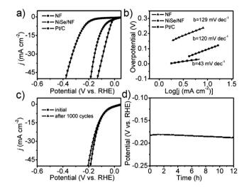
Fig. 7 (a) HER LSVs of NiSe/NF, NF and Pt/C in 1 M KOH. (b) Tafel slopes of the same. (c) LSVs of NiSe/NF before and after 1000 cycles. (d) CA response of the same in 1 M KOH (NF denotes Ni foam). Reproduced with permission from ref. 69 (Copyright 2105 Wiley Publications).
