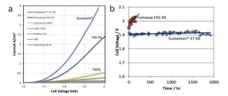
Fig. 9 (a) Comparison of current-voltage response of AEM electrolysis with various membranes in ref. 119. (b) Steady state voltage performance at 1 A cm<sup>-2</sup> with Sustainion 37–50 membrane and FAS-50 membrane (60 °C, 1 M KOH, NiFe<sub>2</sub>O<sub>4</sub> anode and NiFeCo cathode). Reprinted from ref. 125 with permission from Elsevier. 125
