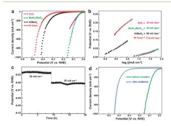
Fig. 2 (a) LSV curves for Pt/C, Ni foam, NiMoO<sub>4</sub>, and MoNi<sub>4</sub>/MoO<sub>3-x</sub>. (b) The corresponding Tafel plots. (c) Short-term stability test of MoNi<sub>4</sub>/  $MoO_{3-x}$ . (d) LSV curves of  $MoNi_4/MoO_{3-x}$  for HER before and after electrochemical oxidation.<sup>38</sup> Reprinted from ref. 38 with permission from John Wiley and Sons.
