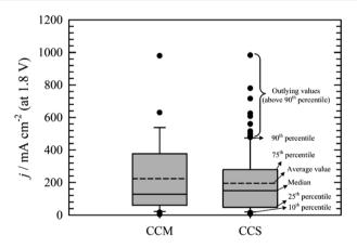
Fig. 6 Comparison of the current densities achieved at cell voltage 1.8 V using the CCM $^{57,59,106,107,114,116,131-136,139-141}$  or CCS $^{22,54,55,95,101-104,108,109,111-113,115,117-124,126-129,142,143}$  method of MEA construction.
