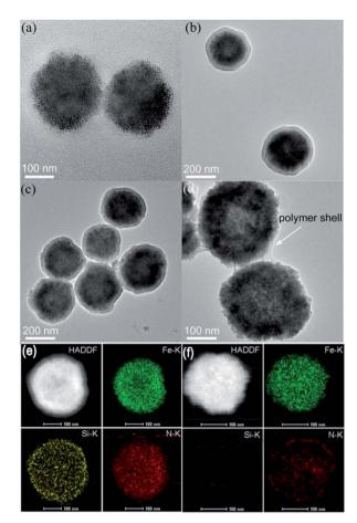
Fig. 1 TEM images of (a) Fe $_3O_4$  NPs, (b) Fe $_3O_4$ @SiO $_2$ , (c) Fe $_3O_4$ @-SiO $_2$ @Poly( $_1$ -Trp), and (d) yolk-shell Fe $_3$ O $_4$ @Poly( $_1$ -Trp). (e) and (f) show the TEM elemental mapping images of Fe $_3$ O $_4$ @SiO $_2$ @Poly( $_1$ -Trp) and yolk-shell Fe $_3$ O $_4$ @Poly( $_1$ -Trp), respectively.
