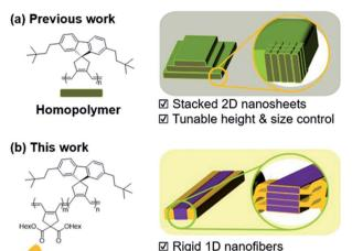
Scheme 1 New strategy to prepare 1D nanofibers with tunable widths and lengths *via* rapid self-assembly.
