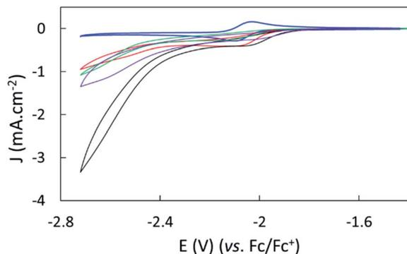
Fig. 3 Cyclic voltammograms of 1 mM complex **1** with 0.1 M TBAPF<sub>6</sub> in dry CH<sub>3</sub>CN on a GC electrode under Ar (blue), CO<sub>2</sub> (red), CO<sub>2</sub> with 0.1 M TFE (black), CO<sub>2</sub> with 0.1 M H<sub>2</sub>O (green) and CO<sub>2</sub> with 0.1 M PhOH (purple). The scan rate was 50 mV s<sup>-1</sup>; the second scan is shown.
