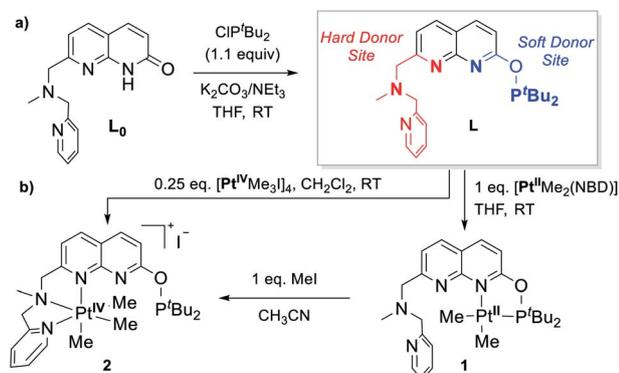
Scheme 2 (a) Synthesis of ligand L; (b) selective binding to Pt<sup>II</sup> and Pt<sup>IV</sup> centers *via* hard and soft sites.
