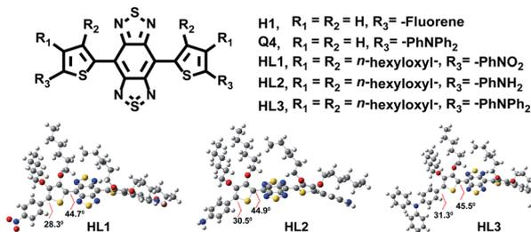
Fig. 1 The chemical structure and optimized ground state geometries (S<sub>0</sub>) of **HL1–HL3** by using the Gaussian 09 software.
