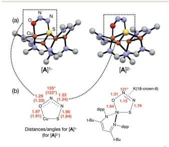
Fig. 2 (a) Optimized structures of N<sub>2</sub>O-activated intermediates [A]<sup>1-</sup> and [A]<sup>2-</sup> (color code: Cu, orange; S, yellow; O, red; N, blue; C, gray). (b) Comparison of the cyclic core structures of  $[A]^{n-}$  and a related mononuclear Ni complex characterized by Hayton;<sup>25</sup> distances are given in Å.
