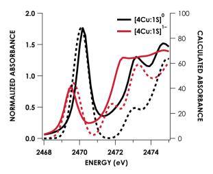
Fig. 6 Overlay of TDDFT-calculated (dashed) S K-edge XAS with experimental (solid) spectra obtained for the [4Cu:1S]<sup>0/1-</sup> redox series. TDDFT calculations were initiated from B3LYP single-point calculations with the CP(PPP)<sup>34</sup> basis set on Cu and the ZORA-def2-TZVP(-f)<sup>38</sup> basis set on all other atoms. Calculated spectra are shifted by +40.4 eV to correct for inaccurate core potential modeling endemic to standard hybrid DFT calculations.
