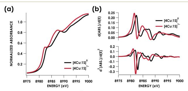
Fig. 3 (a) Cu K-edge XAS spectra obtained for the  $[4\text{Cu}:1\text{S}]^{0/1-}$  redox couple. (b) First (top) and second (bottom) derivative Cu K-edge XAS spectra. Isoenergetic pre-edge (1s  $\rightarrow$  3d) excitations are evident in the second-derivative spectra at 8979.8 eV. Rising edge inflection points occur at 8982.3 and 8985.9 eV for  $[4\text{Cu}:1\text{S}]^0$  and 8981.5 and 8984.8 eV for  $[4\text{Cu}:1\text{S}]^{1-}$ .
