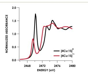
Fig. 4 S K-edge XAS data obtained for the  $[4\text{Cu}:1\text{S}]^{0/1-}$  redox couple. Pre-edge peaks corresponding to S 1s  $\rightarrow \psi^*$  excitations are located at 2470.2 eV for  $[4\text{Cu}:1\text{S}]^0$  and 2469.5 eV for  $[4\text{Cu}:1\text{S}]^{1-}$ .
