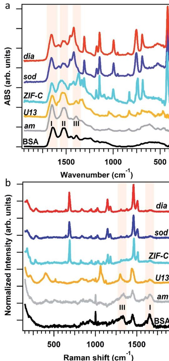
Fig. 3 FTIR (a) and Raman (b) spectra of BSA, the biocomposites with *am*, *dia*, *sod*, *U13* and *ZIF-C* phases. The spectral regions of Amide I, II and III bands of BSA are highlighted in light pink.
