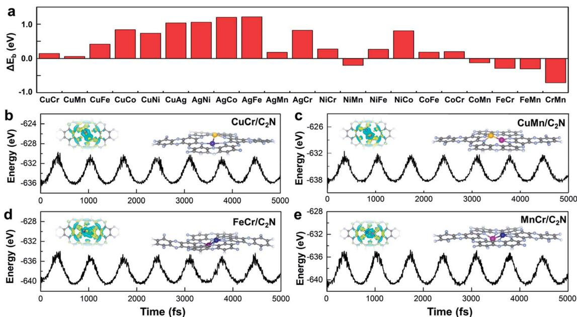
Fig. 2 (a) Energy difference between adsorption energy of TM atoms on  $\text{C}_2\text{N}$  and the cohesive energy of TM atoms. Energy fluctuations of (b) CuCr/ $\text{C}_2\text{N}$ , (c) CuMn/ $\text{C}_2\text{N}$ , (d) FeCr/ $\text{C}_2\text{N}$ , and (e) MnCr/ $\text{C}_2\text{N}$  against the time in AIMD simulations at 400 K. Insets show snapshots of the atomic configuration and charge density difference. Charge depletion and accumulation are displayed in cyan and yellow, respectively.
