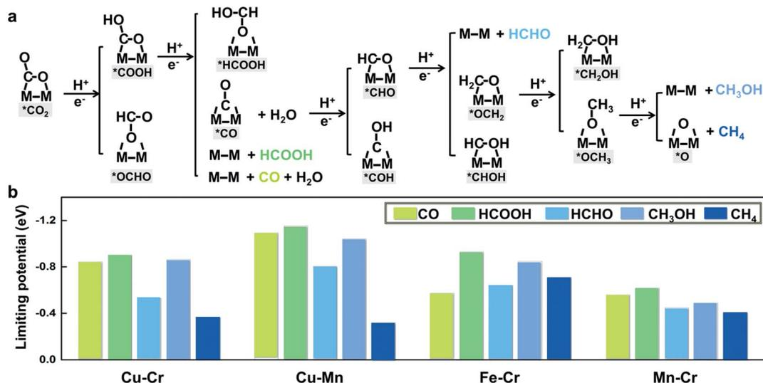
Fig. 4 (a) Schematic depiction of the CO<sub>2</sub> reduction pathways toward a variety of C1 products (CO, HCOOH, HCHO, CH<sub>3</sub>OH and CH<sub>4</sub>) on M<sub>1</sub>M<sub>2</sub>/C<sub>2</sub>N (M<sub>1</sub>M<sub>2</sub> = CuCr, CuMn, FeCr, and MnCr). (b) Thermodynamic limiting potentials toward C1 products (CO, HCOOH, HCHO, CH<sub>3</sub>OH and CH<sub>4</sub>) on CuCr/C<sub>2</sub>N, CuMn/C<sub>2</sub>N, FeCr/C<sub>2</sub>N, and MnCr/C<sub>2</sub>N.
