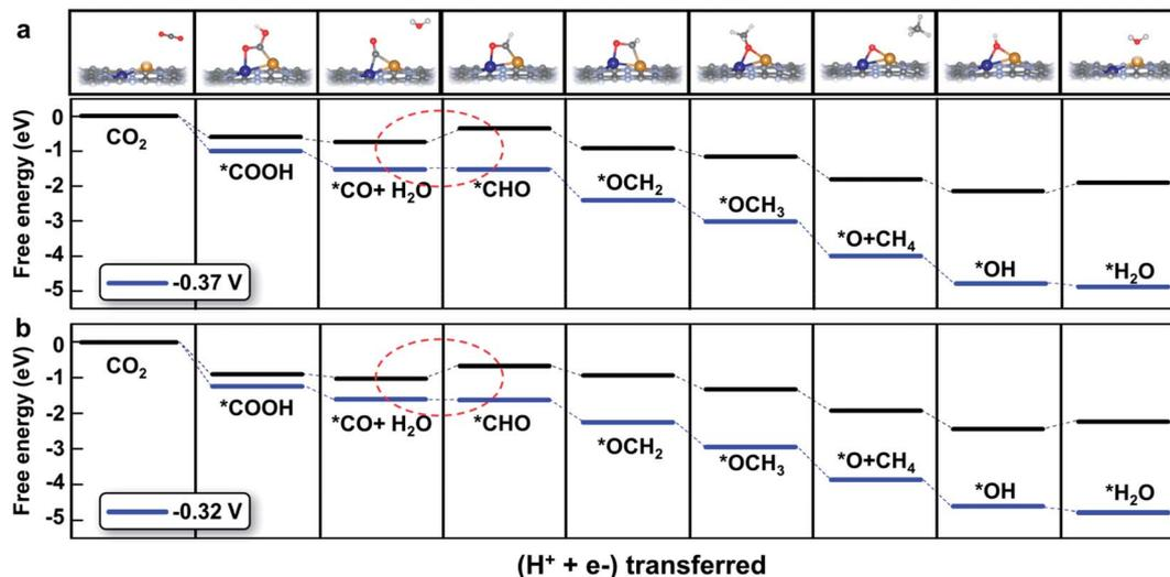
Fig. 5 Free energy diagram of the CO<sub>2</sub> reduction pathway toward CH<sub>4</sub> on (a) CuCr/C<sub>2</sub>N and (b) CuMn/C<sub>2</sub>N at different applied potentials. The potential-limiting steps are marked by red dotted circles.
