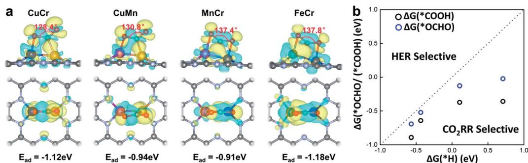
Fig. 3 (a) Side and top views of the charge density difference for CO<sub>2</sub> adsorbed on M<sub>1</sub>M<sub>2</sub>/C<sub>2</sub>N (M<sub>1</sub>M<sub>2</sub> = CuCr, CuMn, FeCr, and MnCr). Charge depletion and accumulation are displayed in cyan and yellow, respectively. (b) Comparison between hydrogen adsorption free energy  $\Delta G(*\text{H})$  and carbon dioxide hydrogenation free energy  $\Delta G(*\text{COOH})/\Delta G(*\text{OCHO})$ .
