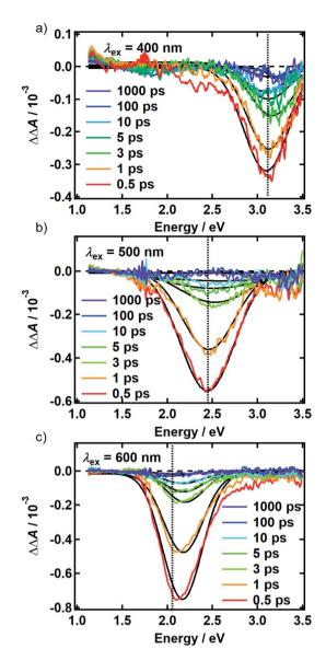
Fig. 4 Time-resolved ground state bleach spectrum isolated from transient absorption spectra recorded using the perpendicular pumpprobe polarizations as described in the text. The spectra are shown for (a) 400 nm, (b) 500 nm, and (c) 600 nm excitation. The photon energy of each pump pulse is indicated by the vertical dashed line. Solid black lines are the Gaussian best fits at each time point.
