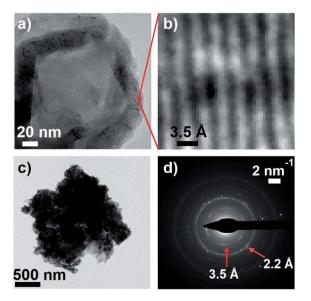
Fig. 9 (a) Transmission electron microscopy (TEM) image of DOPA melanin showing graphite-like stacked layers in the dried material. (b) An expanded view of the indicated region in panel a, showing diffraction. (c) A dense mass of DOPA melanin. (d) The selected area electron diffraction (SAED) pattern from the entire mass in panel c.
