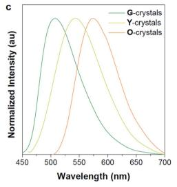
Fig. 1 Structural and optical properties of TPE-EP. (a) D-A based AIE luminogen. (b) Fluorescence photographs of polymorphic G-, Y-, and O-crystals as well as their (c) corresponding emission spectra. Excitation wavelength: 405 nm.
