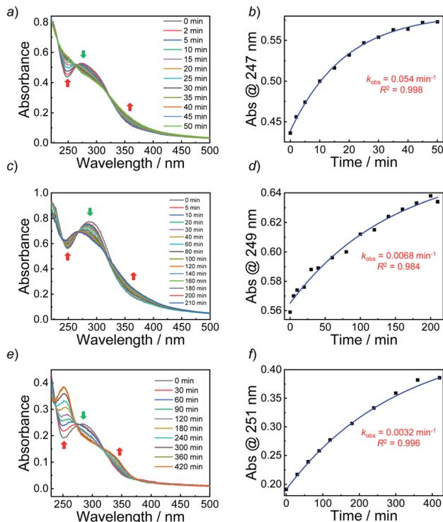
Fig. 4 (a, c and e) Absorbance spectra and (b, d and f) absorbance intensity changes together with a mono-exponential fit of aqueous dispersions ( $0.1 \text{ g L}^{-1}$ ,  $25^\circ \text{C}$ ) of (a and b) **BP1** vesicles, (c and d) **BP2** vesicles, and (e and f) **BP3** micelles under UV 365 nm irradiation ( $4 \text{ mW cm}^{-2}$ ).
