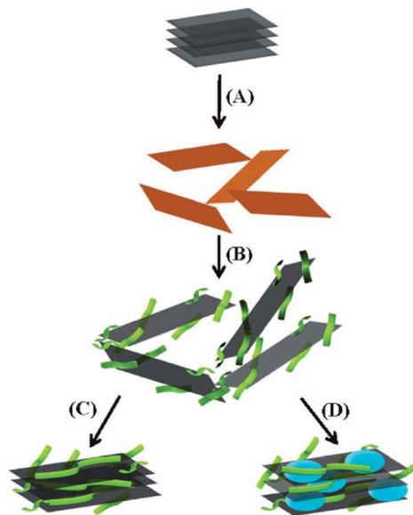
Fig. 14 Schematic illustration of aqueous dispersions of (A) GO, (B) GO-PDI and (C) GO-PyS through  $\pi$ - $\pi$  interaction and (D) co-assembly of negatively charged ssDNA-G sheets and positively charged cytochrome *c* produces co-intercalated multifunctional layered nanocomposites. This figure has been reproduced from ref. 93 with permission from *Adv. Mater.*, Copyright 2009.
