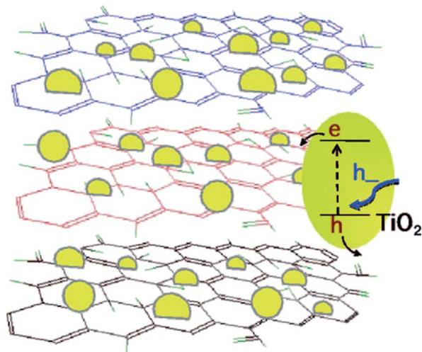
Fig. 7 TiO<sub>2</sub>-graphene composite and its response under UV-excitation. This figure has been reproduced from ref. 69 with permission from *ACS Nano*, Copyright 2008.
