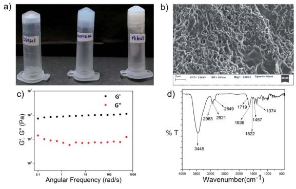
Fig. 8 (a) Gels formed by P1 in kerosene, diesel and petrol, (b) FESEM image of the P1 organogel in kerosene, (c) frequency dependence of the dynamic storage modulus (G') and the loss modulus (G'') of the organogel from P1 in kerosene at 1% w/v. (d) FTIR spectrum of the xerogel of P1 in kerosene.
