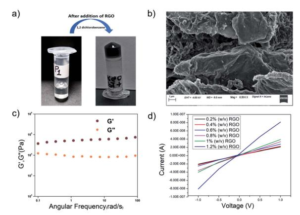
Fig. 10 (a) The reduced graphene oxide incorporated hybrid organogel RGO-P1. (b) An FESEM image of the RGO-P1 hybrid organogel. (c) Frequency dependence of the dynamic storage modulus (G') and the loss modulus (G') of the RGO-P1 hybrid organogel (1 wt%) in 1,2-DCB. (d) I-V curve showing the conductivity of the hybrid organogels upon RGO incorporation.
