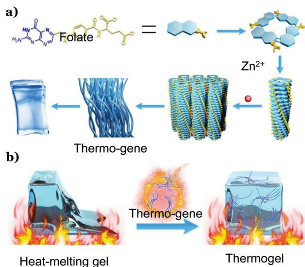
**Scheme 1** Illustration of the folate–Zn<sup>2+</sup> hydrogel thermo-gene (a) and the formation of a thermogel by introducing the thermo-gene into a heat-melting gel (b).
