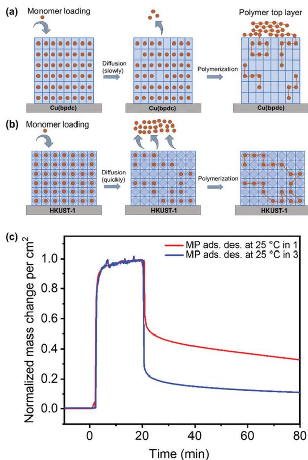
Fig. 4 Schematic diagram showing the depot effect of (a) **MP** diffusion from **1** and (b) quick release from the framework of **3**, followed by polymerization. In (c), the normalized mass change from the adsorption and desorption of **MP** on **1** and **3** measured using a QCM is shown.
