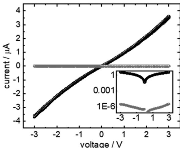
Fig. 7 Conductivity of **polyMP@3**. The current–voltage curve of the **polyMP@3** sample is shown in black, and the current–voltage curve of 3 is shown as a reference in grey. The inset shows the data on a logarithmic scale.
