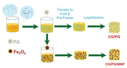
Fig. 1 Schematic illustration of the fabrication procedure of the CG/PG and CG/PG/MNP composite scaffolds.
