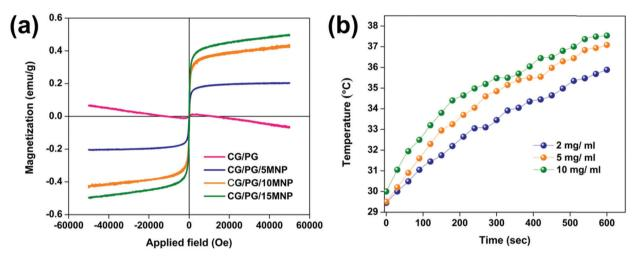
Fig. 6 (a) Hysteresis loop of CG/PG, CG/PG/5MNP, CG/PG/10MNP and CG/PG/15MNP composite scaffolds and (b) the magnetic heating ability of the GC/PG/10MNP composite scaffold evaluated under an alternating magnetic field with different concentrations.
