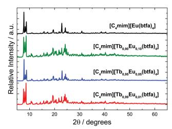
Fig. 2 Powder X-ray diffractograms for the  $[C_4 \text{mim}][\text{Tb}_{1-x}\text{Eu}_x(\text{btfa})_4]$  (x = 0.01, 0.05, 0.10, 1.00) complexes.
