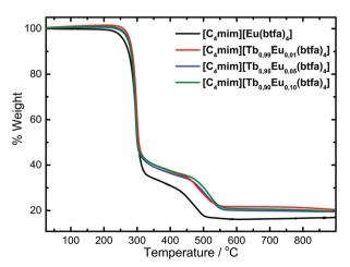
Fig. 1 TGA curves of the  $[C_4 \text{mim}][Tb_{1-x}Eu_x(btfa)_4]$  (x = 0.01, 0.05, 0.10, 1.00) complexes recorded under a synthetic air atmosphere at 10 °C min<sup>-1</sup>.
