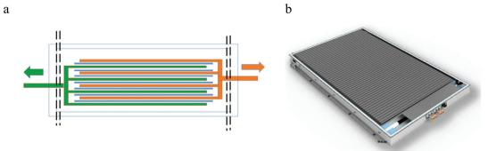
Fig. 7 (a) Schematic diagram showing how opposite tab alignment could simplify cell disassembly (dashed lines show potential cut points), (b) photograph of a BYD pack where lithium ion battery cells (blades) form a structural element of the vehicle and offer easier disassembly.
