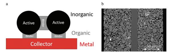
Fig. 8 (a) Schematic diagram of the three component interface in lithium ion batteries, (b) SEM image of an electrode showing that the collectors is ca. 20 µm and the active layers are 20 to 100 µm thick.
