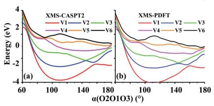
Fig. 8 Six potential energy curves of triplet ozone calculated by (a) XMS-CASPT2 and (b) XMS-PDFT.
