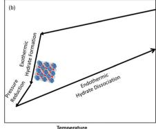
Fig. 27 Two modes of hydrate cold storage technology, namely heating (a) and (b) depressurising for cooling (based on Cheng et al. 920)
