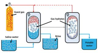
Fig. 28 Schematic diagram of the clathrate hydrate-based desalination process. Seawater is contacted with an appropriate hydrate former such as CO<sub>2</sub> at desired thermodynamic conditions to form clathrate hydrates while excluding salts from the crystalline structure. The hydrate crystal can then be removed from the brine and dissociated to drinking water and hydrate former which could be recycled.
