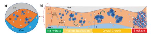
Fig. 14 (a) Schematic model of multiphase flow in pipeline, where hydrate crystal aggregates could flow in gaseous, oleic, and aqueous phases, and/or could deposit onto the pipe solid surface; (b) schematic diagram of the drivers of hydrate crystals formation and aggregation in hydrocarbon transportation pipelines and three-step process of (i) hydrate nucleation, (ii) crystal growth, and (iii) blockage.
