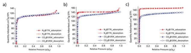
Fig. 2 Gas sorption (blue, CO<sub>2</sub> at 195 K; red, N<sub>2</sub> at 77 K) on three isostructural PCPs: (a) FePzNi (calculated BET surface area using N<sub>2</sub> was found to be  $\sim$  330 m<sup>2</sup> g<sup>-1</sup>), (b) CoPzNi (BET surface area using N $_2\sim$  430 m<sup>2</sup> g<sup>-1</sup>), and (c) NiPzNi (BET surface area using N $_2\sim$ 500 m<sup>2</sup> g<sup>-1</sup>).
