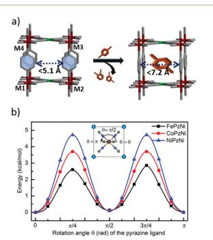
Fig. 4 (a) A schematic representation of the pillar rotation toward the px isomer. (b) The potential energy surface for the rotation of the pyrazine pillars in FePzNi, CoPzNi, and NiPzNi.
