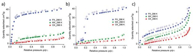
Fig. 3 Pure component xylene isomer (px-blue, mx-green, and ox-red) sorption on the three isostructural PCPs measured at 298 K (a) FePzNi exhibits a typical type-l isotherm for px with an uptake of 40 cm<sup>3</sup> g<sup>-1</sup>. (b) CoPzNi exhibits a stepped profile during the sorption of px with the same uptake as FePzNi. (c) No gate opening was observed for px when using NiPzNi. All three PCPs shown negligible uptake of mx and ox.
