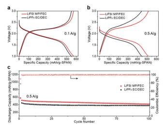
Fig. 2 Li||SPAN half-cell performance in different electrolytes at room temperature. Voltage curves at (a)  $0.1 \,\mathrm{Ag^{-1}}$  and (b)  $0.5 \,\mathrm{Ag^{-1}}$ ; (c) long-term cycling performance at 0.5 A g<sup>-1</sup>.
