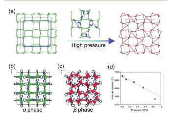
Fig. 18 (a) Scheme of the framework change under high pressure. Crystal structure of ZIF-zni in  $\alpha$  phase (b) and  $\beta$  phase (c). (d) Unit cell volume of ZIF-zni at different temperatures. Partly taken from ref. 123 with
