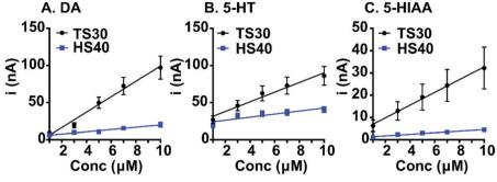
Fig. 3 Sensitivity comparison for TS30 and HS40 fibers. All calibration curves were conducted from 1  $\mu$ M to 10  $\mu$ M. (A) Dopamine (waveform: -0.4 V to 1.3 V, 400 V s<sup>-1</sup>, n = 6-10), (B) 5-HT, and (C) 5-HIAA (waveform for TS30: 0.2 V to 1.0 V, down to -0.1 V and back to 0.2 V, 1000 V s<sup>-1</sup>; HS40: -0.4 V to 1.3 V, 400 V s<sup>-1</sup>, n = 8-10).
