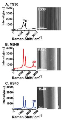
Fig. 1 Example Raman spectra of a standard modulus fiber (TS30, A), intermediate modulus fiber (MS40, B), and high modulus fiber (HS40, C). An SEM image is shown to the right of each spectra. Scale bar is 3  $\mu$ m for each image. The average D/G for each fiber-type is given in Table 1.
