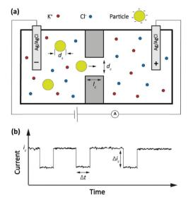
**Fig. 3** (a) Schematic representation of a resistive pulse sensing system. (b) The current transient properties upon particles passing through the pore.
