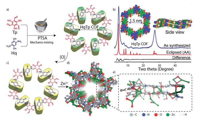
Fig. 1 (a) Schematic representation of the synthesis of HqTp (Hq-2,5-diaminohydroquinone, Tp-1,3,5-triformylphloroglucinol). (b) Powder Xray diffraction pattern with the AA eclipsed slipped SCC-DFT model. (c) The electrochemical oxidation of hydroquinone to quinone in HqTp (d and e). The DFTB model of interlayer interaction of Zn<sup>2+</sup> cations with the adjacent layers of HqTp.
