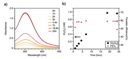
Fig. 2 (a) Absorbance of triiodide (generated from reaction with  $H_2O_2$ ) at different time (0 h, 1 h, 2 h, 3 h, 4.4 h, 7 h, 18.6 h, 24 h). (b) Concentration of  $H_2O_2$  from titrations and corresponding faradaic efficiency during bulk electrolysis with applied bias at 0.42 V vs. RHE under 1 sun light illumination.
