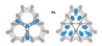
Fig. 3 Schematic representation of possible locations of the Keggin-type  $[PW_{12}O_{40}]^{3-}$  units in the NU-1000 MOF. Colour code: W, blue; P, pink polyhedra; Zr, green; P, pink; C, gray; O, red spheres. Adapted from ref. 40 with permission from The Royal Society of Chemistry.
