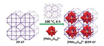
Fig. 4 Schematic depiction of the synthetic procedure used for the preparation of the hybrid [PMo<sub>12</sub>O<sub>40</sub>]<sup>3</sup>-@ZIF-67. Colour code: W, red polyhedra; P, blue spheres. Adapted from ref. 41, with permission from The Royal Society of Chemistry.
