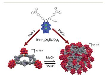
Fig. 8 Schematic illustration of the formation of two types of nanostructures by complexation of  $TBA_6[P_2W_{17}O_{61}(O(Si-C_{29}H_{18}N_3)_2)]_3$  with  $Fe^{2+}$  ions. Colour code: W, blue polyhedra or spheres; P, green polyhedra; Si, yellow; N, violet; C, gray; O, red spheres. Adapted with permission from ref. 54. Copyright 2016 American Chemical Society.
