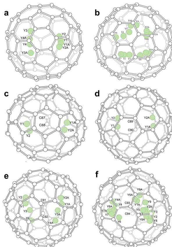
Fig. 1 Perspective drawings showing the internal yttrium sites. (a) 8 in  $Y_2@C_s(6)-C_{82}$ , (b) 14 in  $Y_2@C_{3v}(8)-C_{82}$ , (c) 4 in  $Y_2C_2@C_s(15)-C_{86}$ , (d) 4 in  $Y_2C_2@C_1(26)-C_{88}$ , (e) 8 in  $Y_2C_2@C_2(41)-C_{90}$ , and (f) 17 in  $Y_2C_2@C_2(61)-C_{92}$ .
