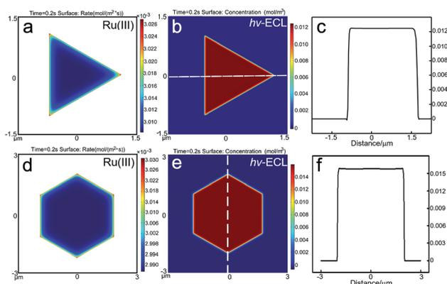
Fig. 3 Results of the simulated reaction rate and concentration profiles. The generation rate of  $\text{Ru}(\text{III})$  on the gold (a) triangular and (d) hexagonal nanoplates. The ECL spatial intensity distribution on the gold (b) triangular and (e) hexagonal nanoplates. (c and f) The distribution of ECL intensity at the measuring line marked in (b and e).
