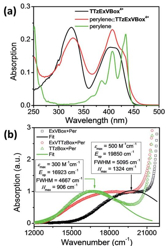
Fig. 3 (a) Steady-state absorption spectra of TTzExVBox<sup>4+</sup>, Per and Per c TTzExVBox<sup>4+</sup> in CH<sub>3</sub>CN. The concentration of Per in the latter two solutions is kept the same. (b) CT bands in Per c ExVBox<sup>4+</sup>, Per c TTzBox<sup>4+</sup>, and Per c TTzExVBox<sup>4+</sup>, and extracted couplings.
