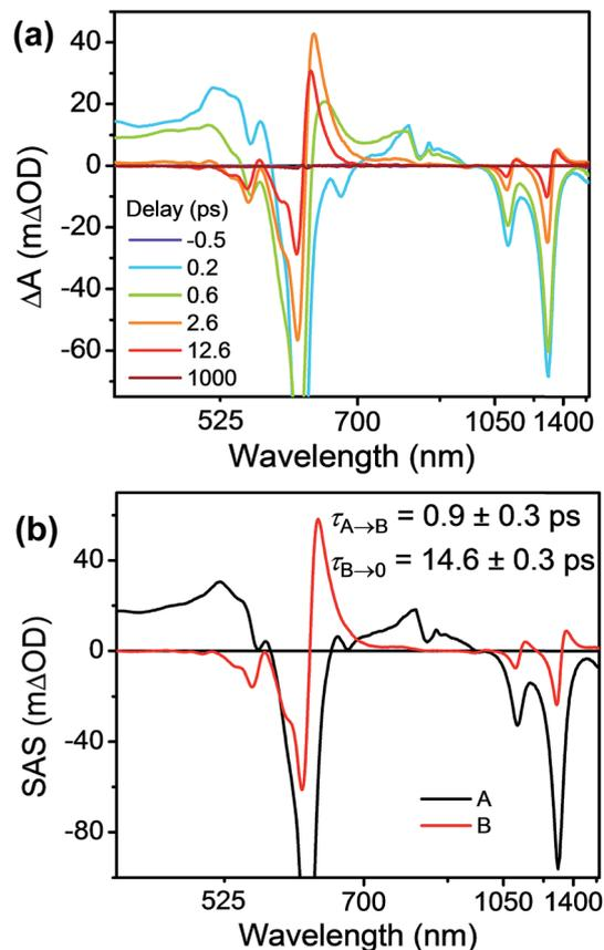
Fig. 6 (a) fsTA spectra and (b) species-associated spectra (SAS) of  $\text{Bn-TTz}^{2+}$  in  $\text{CH}_3\text{CN}$  excited at 620 nm ((A)  ${}^2*\text{TTz}^{2+}$  ( $D_n$ ), (B)  ${}^2*\text{TTz}^{2+}$  ( $D_1$ )). The wavelength axis is plotted in reciprocal space. Time constants are for the representative data set shown here; averages and standard deviations from multiple experiments are given in Table 1.
