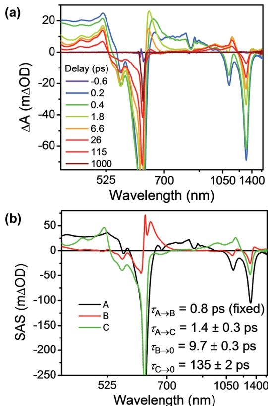
Fig. 7 (a) fsTA spectra and (b) species-associated spectra (SAS) of TTzExVBox<sup>3+</sup> in CH<sub>3</sub>CN excited at 620 nm ((A) <sup>2</sup>\*TTz<sup>2+</sup> (D<sub>n</sub>), (B) <sup>2</sup>\*TTz<sup>2+</sup> (D<sub>1</sub>), (C) TTz<sup>2+</sup>-ExV<sup>+</sup>). The wavelength axis is plotted in reciprocal space. Time constants are for the representative data set shown here; averages and standard deviations from multiple experiments are given in Table 1.
