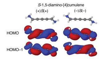
Fig. 4 HOMO and HOMO-1 of (+)S(+) and (-)S(-) conformations S-1,5-diamino-[4]cumulene. The HOMO of (+)S(+) is an M-helix and the HOMO-1 is a P-helix; the order is reversed for the (-)S(-) conformation.
