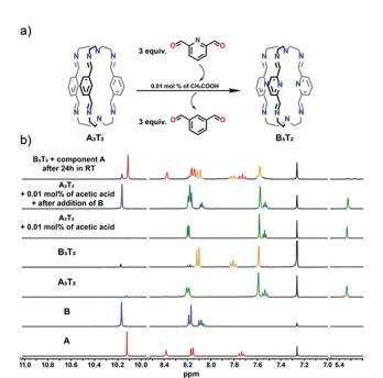
Fig. 6 (a) General scheme of the exchange experiment ( $A_3T_2 + B \rightarrow B_3T_2 + A$ ) between components A + B + T; (b)  $^1H$  NMR spectra of acid catalysed exchange experiment between cage  $A_3T_2$  and component B. For comparison  $^1H$  NMR spectra of components A and B as well as isolated cages  $A_3T_2$  and  $B_3T_2$  are also shown. All NMR spectra were recorded at room temperature in CDCl<sub>3</sub>.
