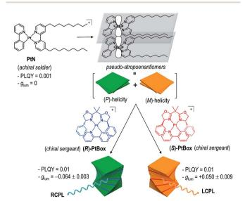
Fig. 1 Molecular strategy to obtaining circularly polarized phosphorescence from superhelical co-assemblies consisting of PtN soldiers and PtBox sergeants.
