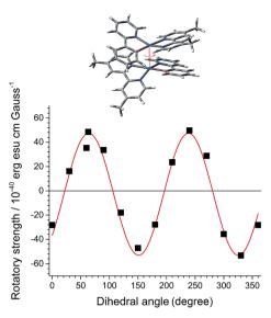
**Fig. 2** Torsional control of chiroptical properties. Simulation of the rotatory strength (*R*) of the MMLCT transition as a function of the dihedral angle of a dimer comprising a truncated form of the PtN molecules (top structure). The red oscillatory curve provides a visual guide. Calculation conditions: TD-CAM-B3LYP/LANL2DZ:6-311+G(d,p)//CAM-B3LYP/LANL2DZ:6-311+G(d,p). Twenty states were considered for the TD-DFT calculations.
