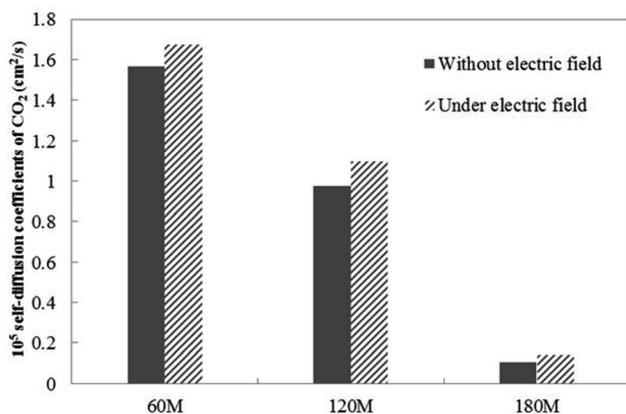
Fig. 4 The CO<sub>2</sub> self-diffusion coefficient of systems in which different amounts of gas molecules are dissolved without an external electric field and under an external electric field.
