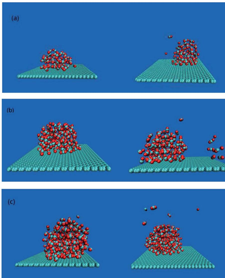
Fig. 2 Snapshot of bubbles under different systems. (a), (b) and (c) are bubbles formed by a system containing 60, 120 and 180 CO<sub>2</sub> molecules respectively, the left side is a bubble without an external electric field, and the right side is a bubble under an external electric field.
