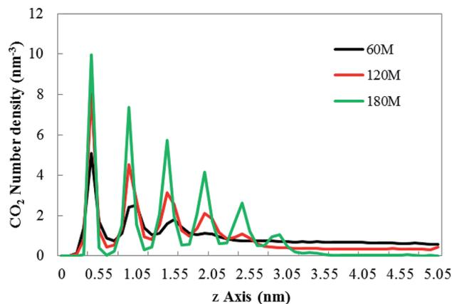
Fig. 3 The CO<sub>2</sub> density profile along the z axis under no external electric field. "60M", "120M", "180M" represent system models containing 60, 120 and 180 CO<sub>2</sub> molecules in this paper, respectively.
