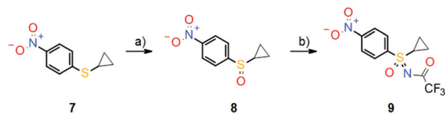
Scheme 4 Synthesis of key sulfoximine building block 9 by rhodium-catalyzed imination of sulfoxide 8 . Reagents and conditions: (a) H_5IO_6 , FeCl_3 , MeCN, rt, 76%; (b) CF_3C(O)NH_2 , PhI(OAc)_2 , MgO, [Rh_2(OAc)_4] , DCM, rt, 78%.
