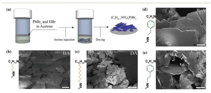
Fig. 1 (a) Schematic diagram of the facile fabrication process of the layered perovskite by injecting a primary amine to a mixture of PbBr<sub>2</sub> in HBr and acetone. (b–e) SEM images of the produced platelets when using short and long aliphatic molecules, such as butylammonium (BA) (b) and decylammonium (DA) (c), and aromatic ones as benzylammonium (BZA) (d) and phenethylammonium (PEA) (e). Scale bars: 100  $\mu$ m.
