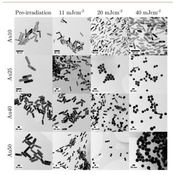
Fig. 4 TEM images taken for each sized AuNR at specific points in the study: before laser irradiation, and after 20 pulses at 11 mJ cm<sup>-2</sup>, 20 mJ cm $^{-2}$ , and 40 mJ cm $^{-2}$ . Scale bars = 50 nm.
