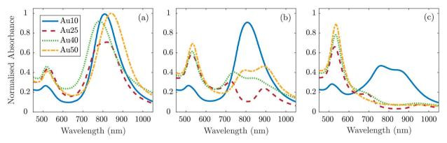
Fig. 5 Absorbance measurements normalised to the maximum of the absorbance spectra taken before laser irradiation (Fig. 1a) for each AuNR size at a concentration of  $1 \times 10^{11}$  NP ml $^{-1}$  after exposure to 20 laser pulses at a fluence of (a)  $11 \pm 1.7$  mJ cm $^{-2}$ , (b)  $20 \pm 2.2$  mJ cm $^{-2}$ , and (c)  $40 \pm 2.6$  mJ cm $^{-2}$ .
