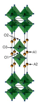
Fig. 1 Crystal structure of the ideal  $A_3B_2O_7$  n=2 RP phase. Atom coordinates used are for air-annealed x=0.75.
