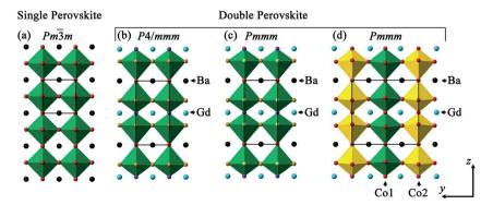
Fig. 1 Crystal structure representation of (a) single  $ABO_3$  perovskite where A is represented in black and  $BO_6$  polyhedra in green; and (b–d) double perovskite  $GdBaCo_2O_6$  where  $Gd^{3+}$  (blue) and  $Ba^{2+}$  cations (black) are ordered in z direction with (b) tetragonal P4/mmm, (c) orthorhombic Pmmm and (d) Pmmm with additional ordered cations along b depicted by  $Co1O_6$  (green) and  $Co2O_6$  (yellow) octahedra ordering.
