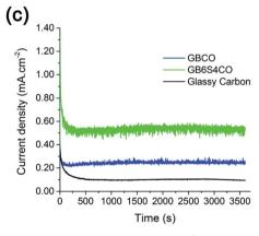
Fig. 9 (a) Linear sweep voltammetry at the 6<sup>th</sup> cycle and the corresponding (b) Tafel plot (at 1 mV s<sup>-1</sup> scan rate) in 0.1 M KOH electrolyte. Chronoamperometry measurements of different GBSCO compounds at 1.65 V ( $\eta = 420$  mV). Electrochemical measurements were iR compensated using current interrupt method. Higher performance was achieved with higher Sr dopant level.
